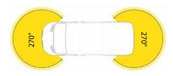
With the Hänsch HT solutions, you can provide the legally required geometric visibility even if the mounting of conventional beacons is not possible due to the structural conditions.
